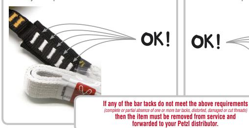
4 - At the harness end, check on each side of the webbing that there are **4** black bar tacks connecting the tear webbing to the black attachment loop.
