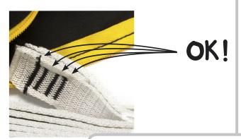
4 - At the harness end, check on each side of the webbing that there are **4** black bar tacks connecting the tear webbing to the attachment loop.
