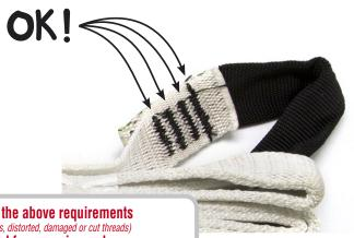
If any of the bar tacks do not meet the above requirements (complete or partial absence of one or more bar tacks, distorted, damaged or cut threads) then the item must be removed from service and forwarded to your Petzl distributor.
